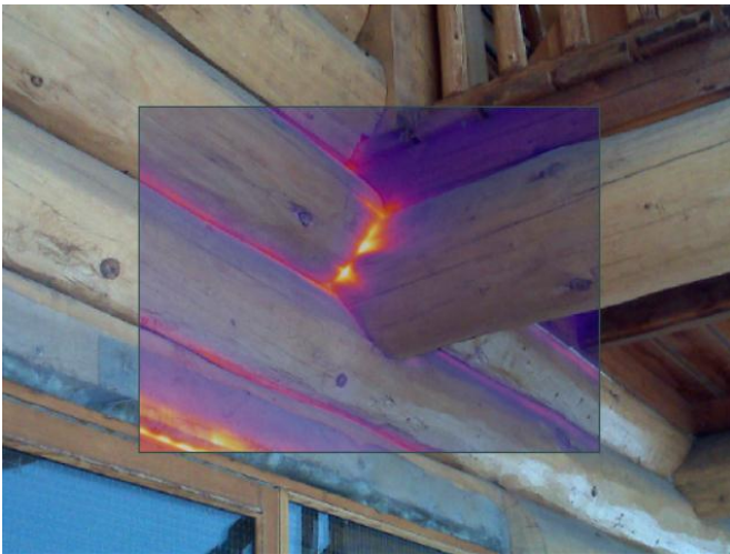
Fig.3.15 Air leakage at joints under pressurization.
