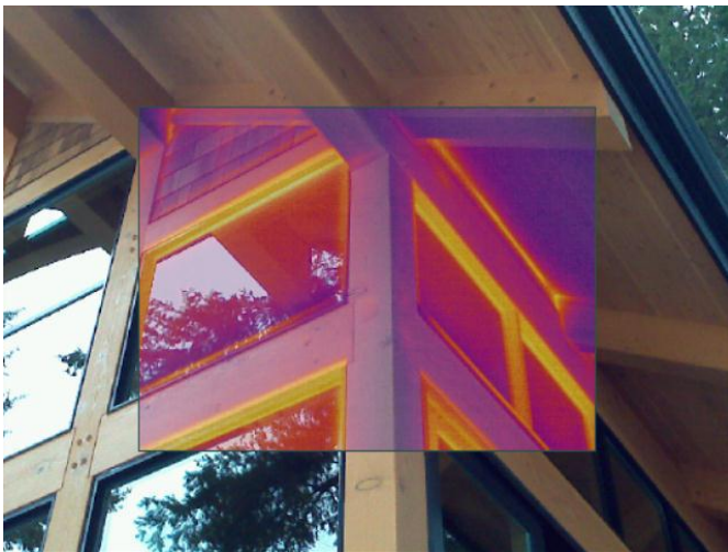
Fig.3.23 IR photo of the roof to wall interface during depressurization (left) and pressurization (right), showing air leakage at this interface during pressurization.
