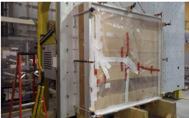
Fig.2.1 Front view of Cascadia Windows in-house Test Wall
