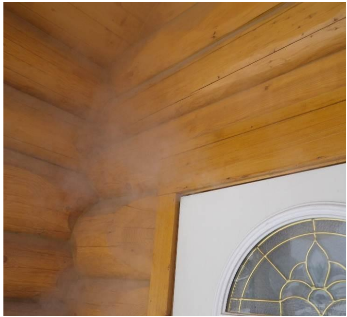
Fig.3.5 Smoke infiltration observed at corner joints and exterior door during smoke testing from the interior under pressurization.
