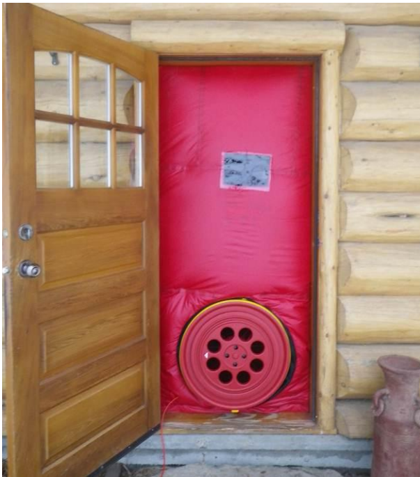
Fig.3.1 Blower door test apparatus viewed from the exterior (left) and the interior (right).
