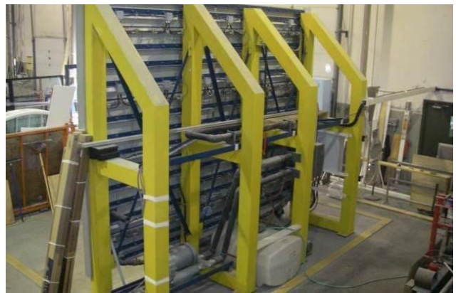
Fig.2.2 Rear view of Cascadia Windows in-house Test Wall
