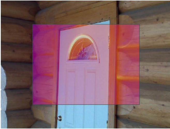
Fig.3.6 IR photo of the door during depressurization (left) and pressurization (right), showing air leakage around the door during pressurization.
