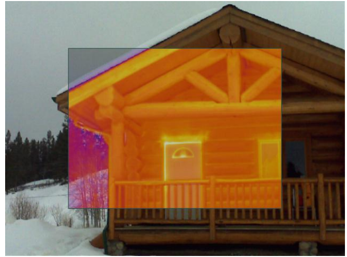
Fig.3.6 IR photo of the door during depressurization (left) and pressurization (right), showing air leakage around the door during pressurization.
